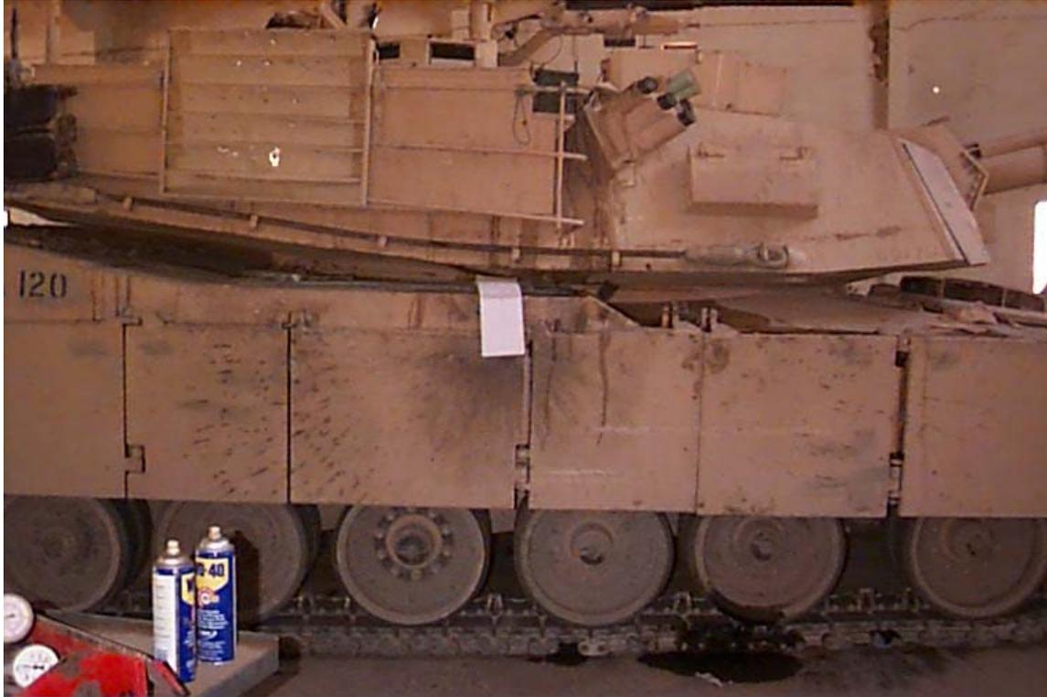
The hole is about the diameter of a pencil. My little finger will not go into it. It is in the skirt proper very near where the bead weld makes a ninety-degree turn to go up for the hinge. On the inside the skin protrudes slightly around the hole. From there the "something" traveled over the track and below the deck entering the hull with the same size hole.
